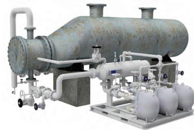
▲ Figure 13. Condensate outlet piping that is 80 in. above grade is preferred, but it is still possible to drain reboilers on low-fill installations with an outlet at 30 in. by using multiple pump/trap units in a package design (as shown here).
