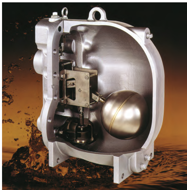
▲ Figure 11. A pump/trap assembly contains a mechanical actuator system. When the reboiler reaches a high level of condensate, the actuator opens a motive valve that inputs high-pressure steam to discharge the condensate.
