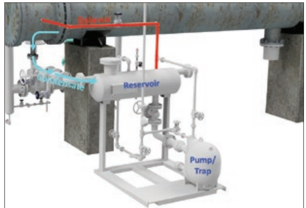
FIGURE 6. A proper condensate vessel balance line is needed so that incoming condensate can displace vapor without increasing vessel pressure
