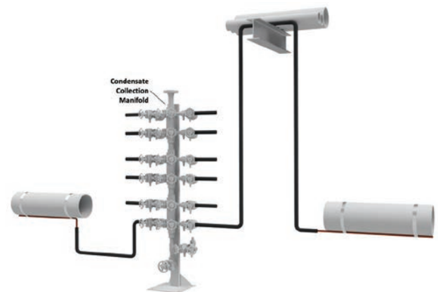
FIG. 6. Tracing systems may require special trap options to mitigate steam locking from uplifts.
