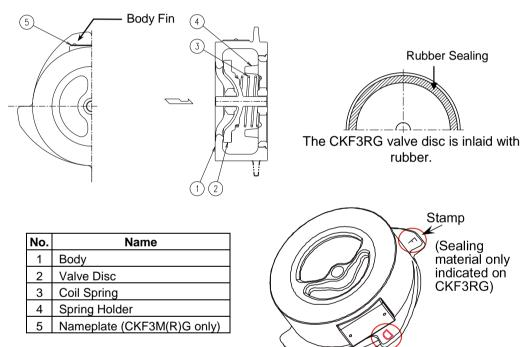
Replacement parts are not available for CKF3 series (flangeless) check valves, as special equipment is required for assembly/disassembly.
