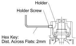
2) Tighten the holder further in with a socket wrench.
