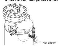
NOTE: Cycle Counter cannot be installed on GP series PowerTraps insulated with an insulation thickness exceeding 40 mm.
