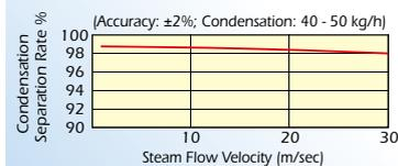
$$\text{Separation Rate(\%)} = \frac{\text{quantity of condensate discharged}}{\text{quantity of incoming condensate}} \times 100$$
