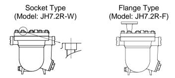
In principle, steam traps automatically discharge inflowing condensate. However, if low-temperature condensate in the piping blocks the trap inlet passage, displacement inside the piping of steam by condensate is obstructed and condensate can no longer flow into the trap (steam-locking). Traps only function in the presence of condensate inflow. A pressure-balancing line prevents the occurrence of steam-locking.
