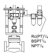
Integrated Filter: 0.3 µm + 5 µm
