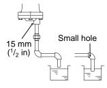
underwater, make sure the piping has a small hole, as shown in the drawing below.
