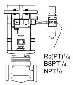
Integrated Filter: 5 µm
