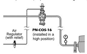
When operating the PN-COS-16 remotely by manual operation, an air regulator (with relief function) that adjusts motive air pressure is required. Adjust the set pressure with the air regulator while checking the pressure gauge on the secondary side.
