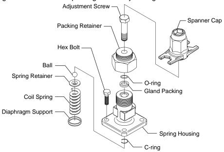
NOTE: Make sure that there are no scratches or wear on the internal parts. Do not reuse the O-ring and the gland packing.
