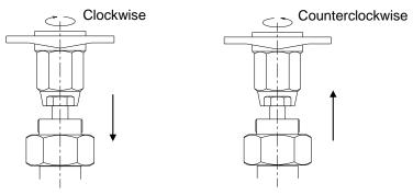
Tighten the adjustment screw to increase pressure
