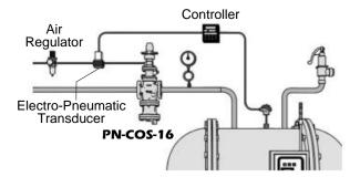
Automatic control is possible when the PN-COS-16 is used with a controller. However, an electro-pneumatic transducer is required in order to control the air for operation. The wiring, etc. should be carried out according to the instruction manual for the controller, the electro-pneumatic transducer, or related devices.
