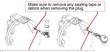
Make sure to install the sensor arm without bending.
