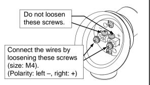
For the terminal box type, wiring is necessary to the terminal box. Before wiring, refer to the "Specifications" section to make sure that the supply power voltage meets these specifications. Make sure that the wires are securely connected to the terminal box using the ring or the spade terminals. Waterproofing of the wiring inlet should be carried out using a waterproof cable gland, etc.
