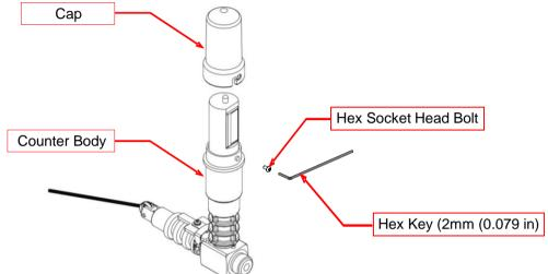
2. Once the cap is removed, turn the silicon-molded LCD display so that the LCD display is readable. After the adjustment is made, put the transparent cap back on and retighten the hex socket head bolt (tightening torque: 0.5 N·m (0.4 lbf·ft)).
