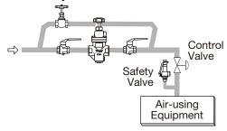
A control valve (i.e. for temperature control) installed between the product and the equipment (downstream of the product) may raise the pressure between the product and the control valve when the control valve is closed, depending on their proximity. Therefore, this valve should be installed close to the air-using equipment, as illustrated. Also, a safety valve should be installed downstream of the control valve.
