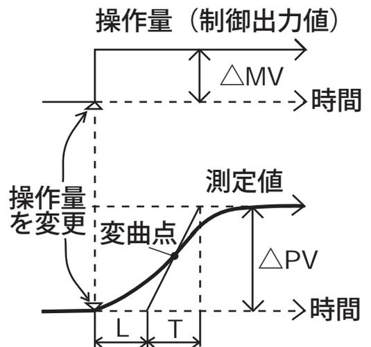
$$K_p = \frac{\Delta PV}{(\text{測定レンジ幅})} \times 100 \times \frac{1}{\Delta MV}$$
