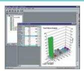
TrapManager processes data from TM5N-EX and then presents the results in a number of ways that users can select. For example, users can tabulate data for specific conditions and calculate the current failure state and rate based on available historical data.
