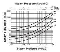
The chart to the left is used to determine the steam flow rate through the DC7 separator. It is based on a steam velocity in the piping of 30 m/s. For other cases, use the equation below and replace "v" with your steam velocity: Effective flow rate
