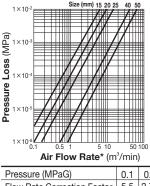
The pressure loss chart is based on an air pressure of 1 MPaG. For other pressures, multiply the air flow rate by the correction factor given in the table below. Use this value on the pressure loss chart.
