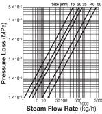
The pressure loss chart is based on a steam pressure of 1.0 MPaG. For other pressures, multiply the steam flow rate by the correction factor given in the table below. Use this value on the pressure loss chart.
