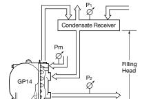
The discharge capacity is determined by the motive medium, motive medium pressure (P<sub>m</sub>) and back pressure (P<sub>2</sub>).
