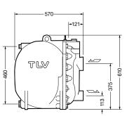
Weight (kg): 124 (Cast Iron), 136 (Cast Steel)
