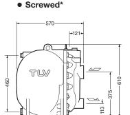
Weight (kg): 127 (Cast Iron), 139 (Cast Steel) \* Rc(PT), other standards available • Flanged\*\*
