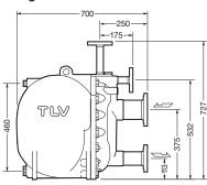
Weight (kg): 149 (Cast Steel) \*\* ASME Class 150 RF, other standards available
