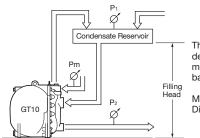
The discharge capacity is determined by the motive medium, motive medium pressure (Pm) and back pressure ( $P_2$ ).
