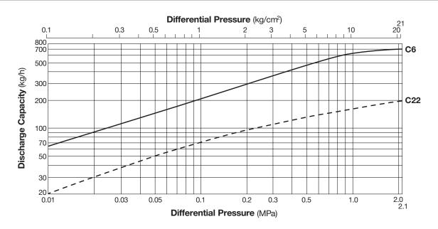
1. Differential pressure is the difference between the inlet and outlet pressure of the trap.
