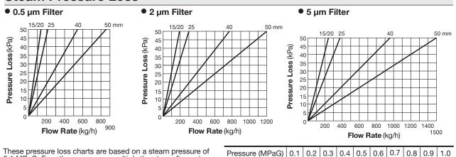
These pressure loss charts are based on a steam pressure of 0.1 MPaG. For other pressures, multiply the steam flow rate by the correction factor given in the table right. Use the result on the pressure loss chart.
