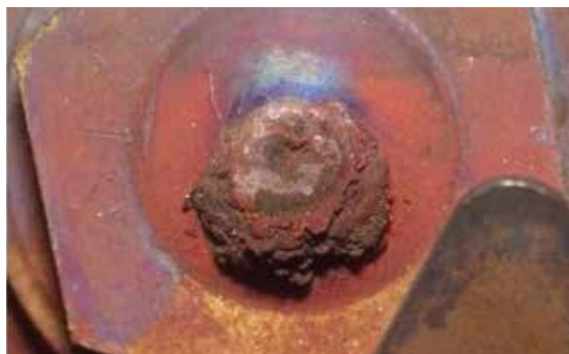
▲ Figure 18. Leached copper from tracing lines can fall out of solution during condensate flashing, build up inside the steam trap, and then block the trap's orifice.
