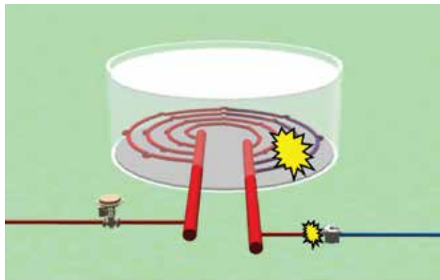
▲ Figure 20. Storage tanks can experience water hammer caused by steam locking when the trap is located on the same plane as the coil outlet.
