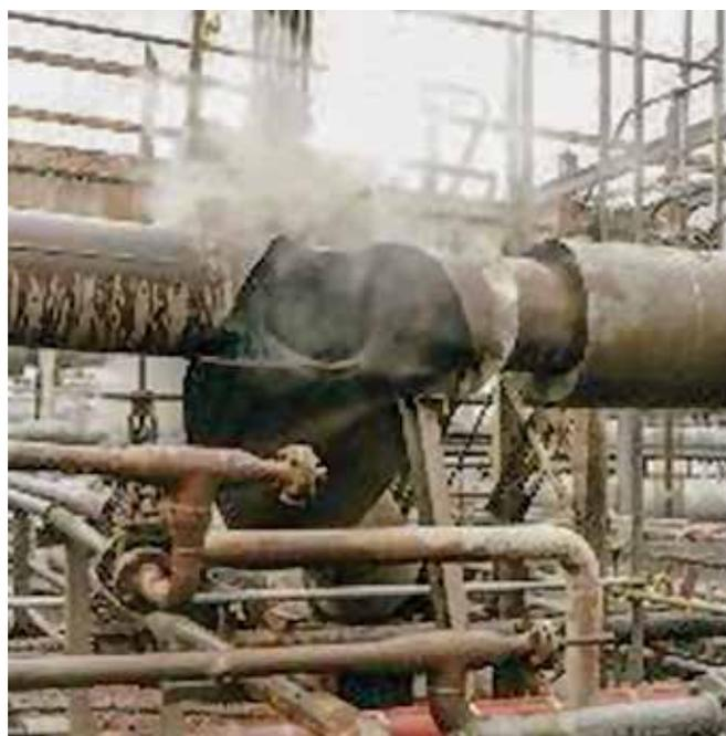
FIG. 2. Failure of a steam pipe joint due to water hammer.
