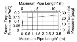
Use the non-freeze valve on a steam trap with an inlet pressure as shown on the graph
