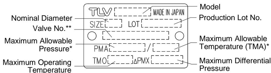
\* Maximum allowable pressure (PMA) and maximum allowable temperature (TMA) are PRESSURE SHELL DESIGN CONDITIONS, **NOT** OPERATING CONDITIONS.
