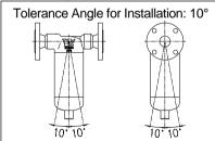
Make sure the product is installed with the raised TLV lettering on the body horizontal.
