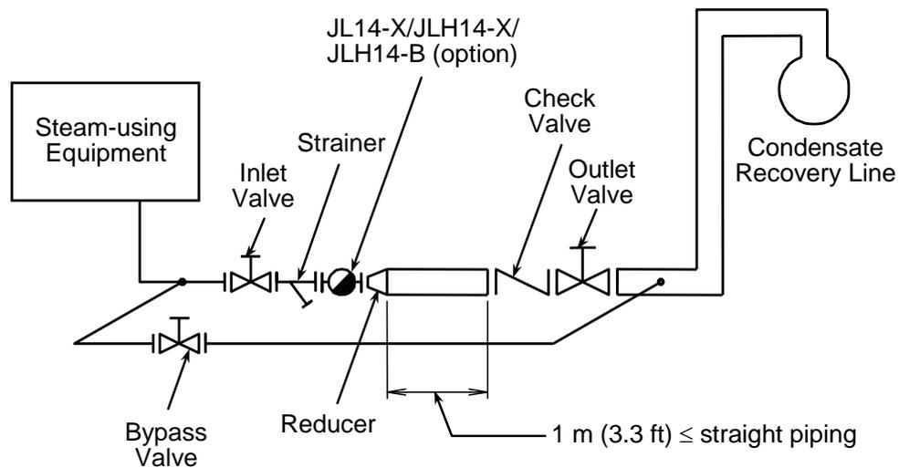
**NOTE:** Be sure to size outlet piping large enough to accommodate any flash steam that may form to prevent any increase in back pressure. (Outlet pipe size should always be properly calculated, contact TLV for assistance.)
