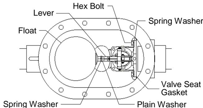
**Detaching / Reattaching the Lever Unit & Float Unit**
