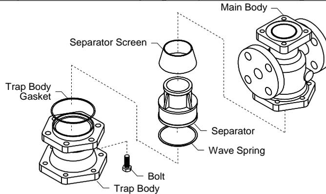
**Removing/Reattaching the Trap and its Components**
