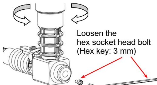
Adjust the counter body by twisting within 15° to the left or right. The angle should be adjusted based on the matching mark on the body.
