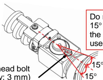
Do not turn the switch unit more than 15° to the left or right. The position of the hex socket head bolt should be used to determine the angle.
