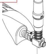
Make sure that the switch unit is facing upwards.
