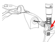
For both the counter unit and terminal box types, use a tool such as an adjustable wrench to grip the square portion of the sensor body (distance across flats: 30 mm) and screw the product in. Applying a force to any part of the product other than the square portion may deform or damage the product.
