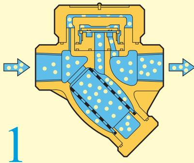
At start-up, the bimetal air vent ring is contracted, lifting the disc off the valve seat and allowing rapid discharge of air and cold condensate.
