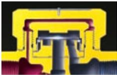
In traps with a single-layer cap, adverse atmospheric conditions and radiant heat loss result in steam loss from no-load actuation and
