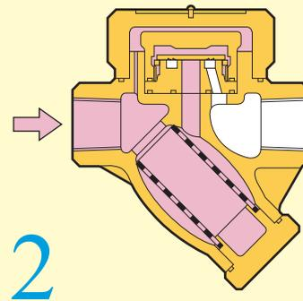
As temperature in the trap rises, the bimetal expands and releases the disc. The disc is forced downward by the low-pressure area created by the rapid flow of flashing condensate/steam below the disc, and the simultaneous high pressure in the pressure chamber above it. A steam jacket insulates the cap's pressure chamber from the radiant heat loss that could cause no-load actuation.
