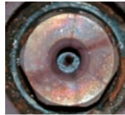
Clogging due to Scale
