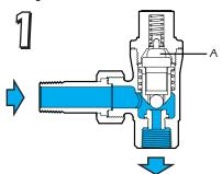
At low temperatures during start-up, the thermo-element (A) is fully retracted, keeping the valve fully open and allowing air and condensate to be discharged.
