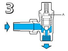
When the temperature of the condensate in the trap drops below approx. 203 °F, the thermo-element (A) retracts, discharging condensate. If the temperature rises above approx. 212 °F, the valve shuts again as in step 2.
