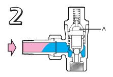
After discharging the initial condensate from start-up, as the condensate temperature raises past approx. 212 °F the thermo-element (A) expands and pushes the valve shut.
