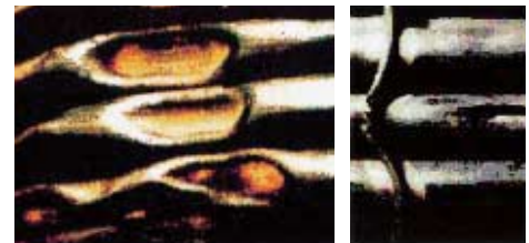
Water hammer damage to tubes and stays
