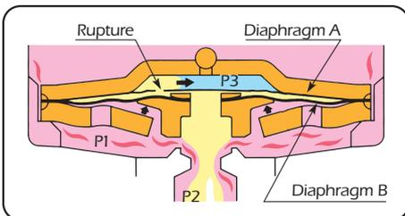
The pressure P3 approaches P2 and the valve plug is pushed up by the primary pressure P1 to open the valve.
