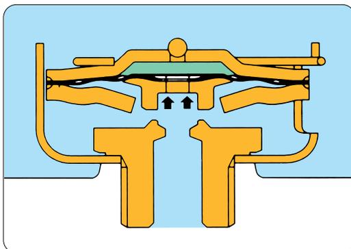
During start up of steam-using equipment while the capsule is still cold, the fill is in liquid state. The internal pressure is lower than the external pressure so that the diaphragm is pushed up to open the valve. Air, gases and condensate are discharged.
