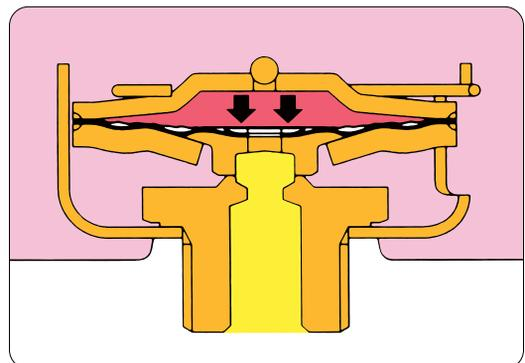
As the condensate temperature approaches steam temperature, the capsule fill boils and evaporates, increasing the internal pressure which expands the diaphragm.
