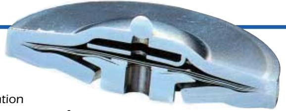
The capsule element contains a liquid whose saturation temperature is slightly lower than the saturation temperature of water. With rising temperature in the trap, the fill evaporates; the resulting internal pressure expands the diaphragm to close the valve. When the temperature decreases, the fill condenses and the resulting pressure reduction allows the diaphragm to contract and open the valve.
