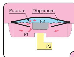
1. When the diaphragm breaks, its fill escapes and the primary pressure P1 builds up in the element above the diaphragm.
