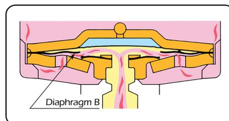
Even in an extreme case, where the valve plug is severed completely from the lower diaphragm, the condensate can drain through the hole in the valve plug center.
