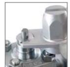
Tightening the gland retainer
