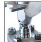
Adjusting the valve aperture
