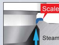
Scale is scraped off and flushed with steam by operating the valve
