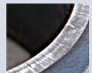
Pipe wall thinning caused by leakage due to valve trim erosion
