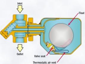
valve off the seat. Instead, the float itself is the valve, and the buoyant force of the condensate serves to "roll" instead of pull the valve off the seat as the level of condensate in the trap rises. The rotational movement of the float valve allows precise opening to perfectly match flow requirements.
