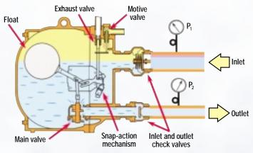
Figure 2. Combination Pump/Trap
