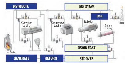
**FIGURE 1.** A steam system has four stages: generate, distribute, use and return of recoverable energy. Equipment performs best with dry steam and when condensate is drained quickly. Recovered energy reduces boiler load
