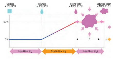
FIGURE 2. Heat energy is needed to change state and elevate temperature. Phase changes occur when ice becomes water and water becomes steam. Steam exits boilers with a certain amount of wetness (3–5%, not saturated)
