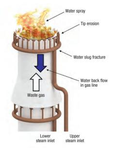
FIGURE 12. Multiple flare issues can be mitigated through proper drainage and operation
