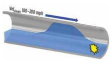
**FIG. 5.** Warning: Condensate level can build up in a steam line when it is not removed, creating a dangerous condition.
