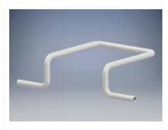
FIG. 10. Danger: Expansion loops on steam lines without a collecting leg to remove condensate can expect water hammer.
