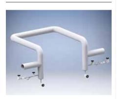
**FIG. 14.** Bi-directional steam flow requires condensate collecting legs/CDLs on both sides of an expansion loop.
