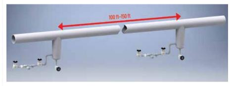
FIG. 9. Collecting legs and CDLs are normally located every 100 ft-150 ft, as well as at risers, drops and before expansion loops.
