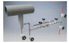
**FIG. 8.** An effective collecting leg/CDL includes a variety of piping components.
