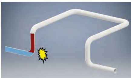
FIG. 20. Vertical loops on CR require the condensate level to build and seal off vertical piping, and hammer is the likely result.
