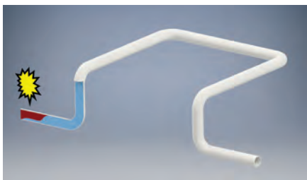
FIG. 21. As condensate rises in a CR vertical loop, some is displaced by low-energy flash steam, which can collapse.
