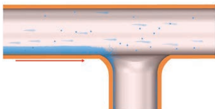
FIG. 5. All steam systems can have condensate flowing along the bottom of the pipe, and moisture is expected in flowing wet steam supply.
