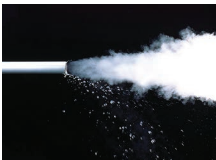
FIG. 4. If not superheated, steam contains substantial moisture that should be disentrained and drained.
