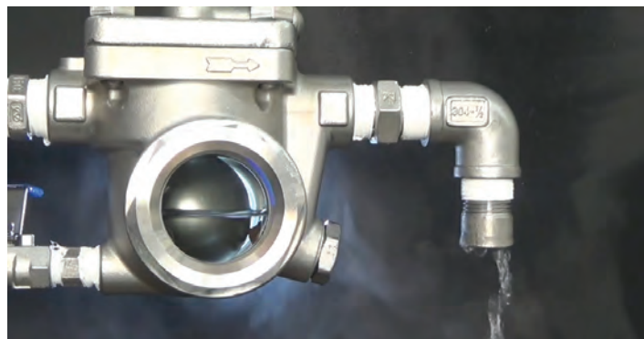
FIG. 4. FT combination trap designs can discharge condensate immediately as it forms.
