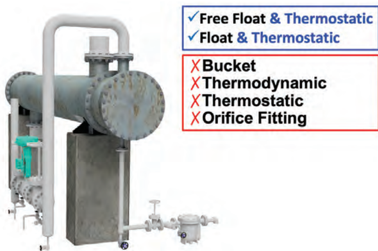
FIG. 3. The author's preference is to use FT or FFT trap models for drainage where suited.
