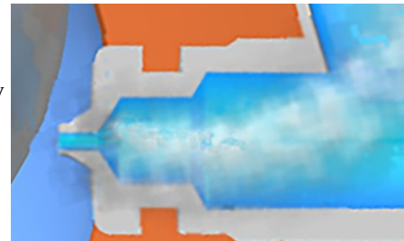
▲ Fig. 7. Light color section represents flash steam from condensate.
