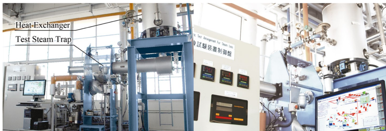
▲ Fig. 8. The test apparatus has been independently validated to comply with ASME PTC39-2005 and ISO 7841 standards.
