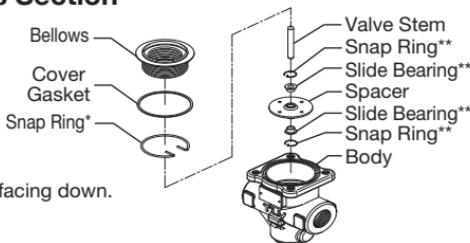
\*\* Cannot be removed individually as it is incorporated with the spacer and must be replaced as a set with the spacer.
