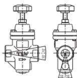
**Make sure the DR20/A-DR20 is installed on horizontal piping with the adjustment handle facing up.** Ensure the raised TLV lettering on the body is horizontal and the arrow is pointing in the direction of flow. The allowable inclination of the DR20/A-DR20 is 10° front-to-back and 15° horizontally.
