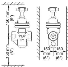
Leave sufficient space for maintenance, inspection and repair.
