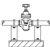
Install the DR20/A-DR20, paying attention to avoid excessive load, bending and vibration. Supporting the inlet and outlet pipes securely is recommended.
