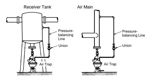
Connect the pressure-balancing line in the following manner:
