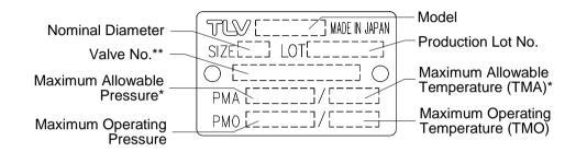
\* Maximum allowable pressure (PMA) and maximum allowable temperature (TMA) are PRESSURE SHELL DESIGN CONDITIONS, **NOT** OPERATING CONDITIONS.
