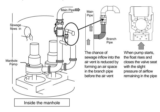
2. The air vent remains open while the manhole pump is stopped, and discharges air that enters the main pipe and pump.
