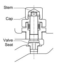
To operate the lock release valve:
