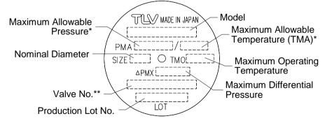
\* Maximum allowable pressure (PMA) and maximum allowable temperature (TMA) are PRESSURE SHELL DESIGN CONDITIONS, **NOT** OPERATING CONDITIONS.
