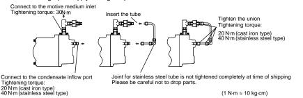
**CAUTION** Using appropriate tools, make sure that the union joint has been tightened properly. Improper tightening may lead to steam leakage, resulting in burns or other injury.
