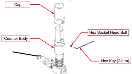
2. Once the cap is removed, turn the silicon-molded LCD display so that the LCD display is readable. After the adjustment is made, put the transparent cap back on and retighten the hex socket head bolt (tightening torque: 0.5 N·m).
