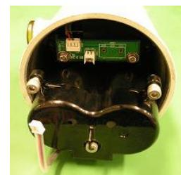
4. Insert a new battery pack and secure it with 2 screws.
