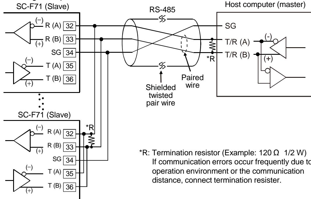
\*R: Termination resistor (Example:  $120\ \Omega$  1/2 W)
