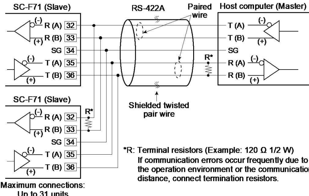
\*R: Terminal resistors (Example: 120 Ω 1/2 W)
