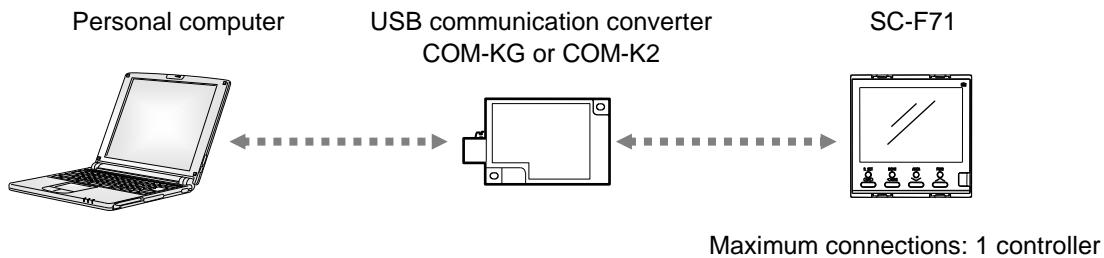
**NOTE** The Loader port is only for parameter setup. Not used for data logging during operation.
