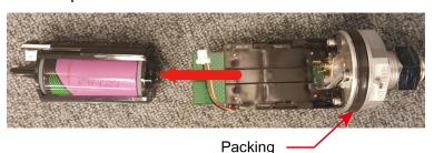
4. Replace the packing and coat surfaces with grease. Insert a new battery pack from above by sliding it along the grooves. Attach it to the connector. Make sure that both left and right guides on the battery pack are in the grooves. Place the cap back on and tighten the cap screw with a hex key, clockwise as viewed from above.
